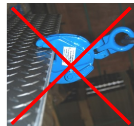
Improper Horizontal Lift
