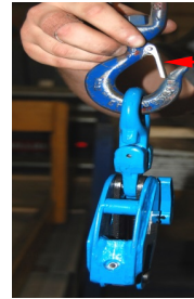
Hook with automatically closing latch
